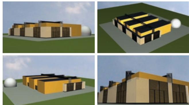
BioGTS® Biogas plant, feedstock 73 000 t/y, 200 t/d of biowaste.
